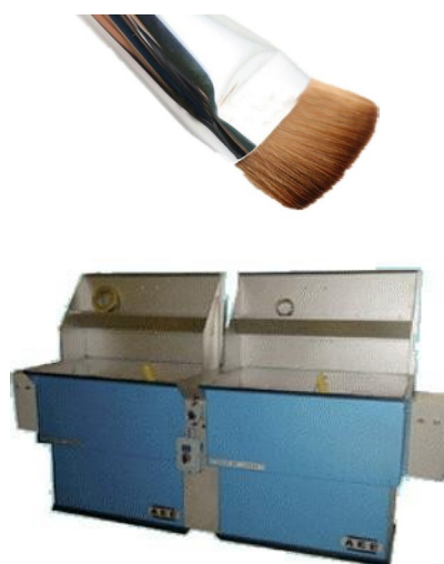
Hot and cold immersion tanks
